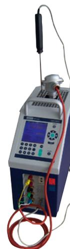
**CTD9300 as an application with an external reference thermometer**
